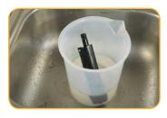
Soak sensor for a minimum of two hours in 140 mg/L ammonium as N standard or the highest standard you plan to use during calibration.
