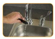
Soak overnight for the best long-term results. Rinse thoroughly with deionized water prior to calibration.
